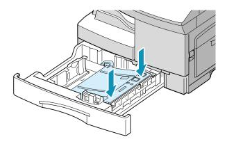
**3** Adjust the rear paper guide to the desired paper length. It is preset to Letter or A4 size depending on country. To load another size, lift and insert the rear guide into the corresponding position.
